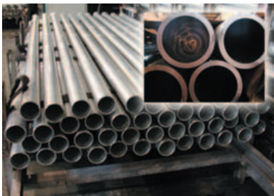
The large diameter and thickness of Easton's start stock allows for ample cold-working while reducing the tubes to final size.
